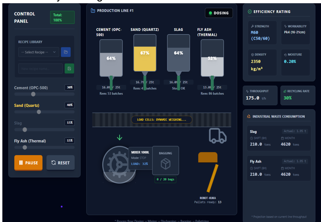
Figure 3- Operation of the digital twin in the dosing mode
