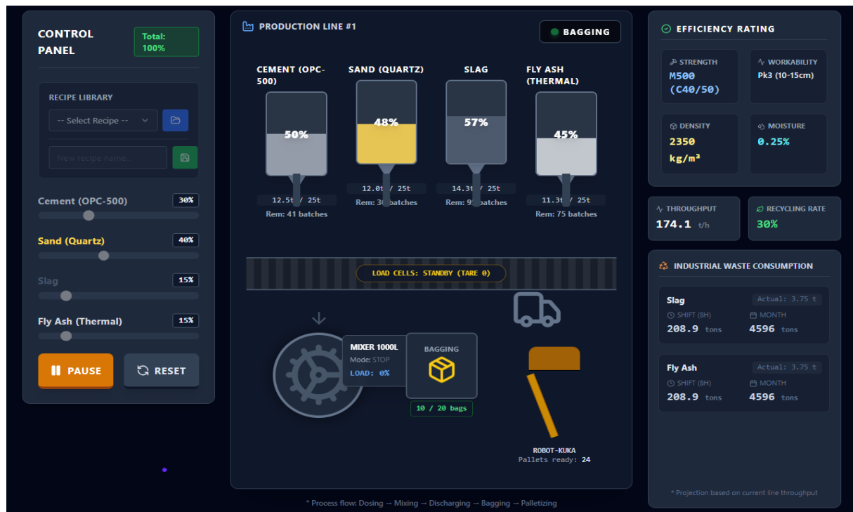
Figure 3- Operation of the digital twin in the mode of loading bags into pallets
